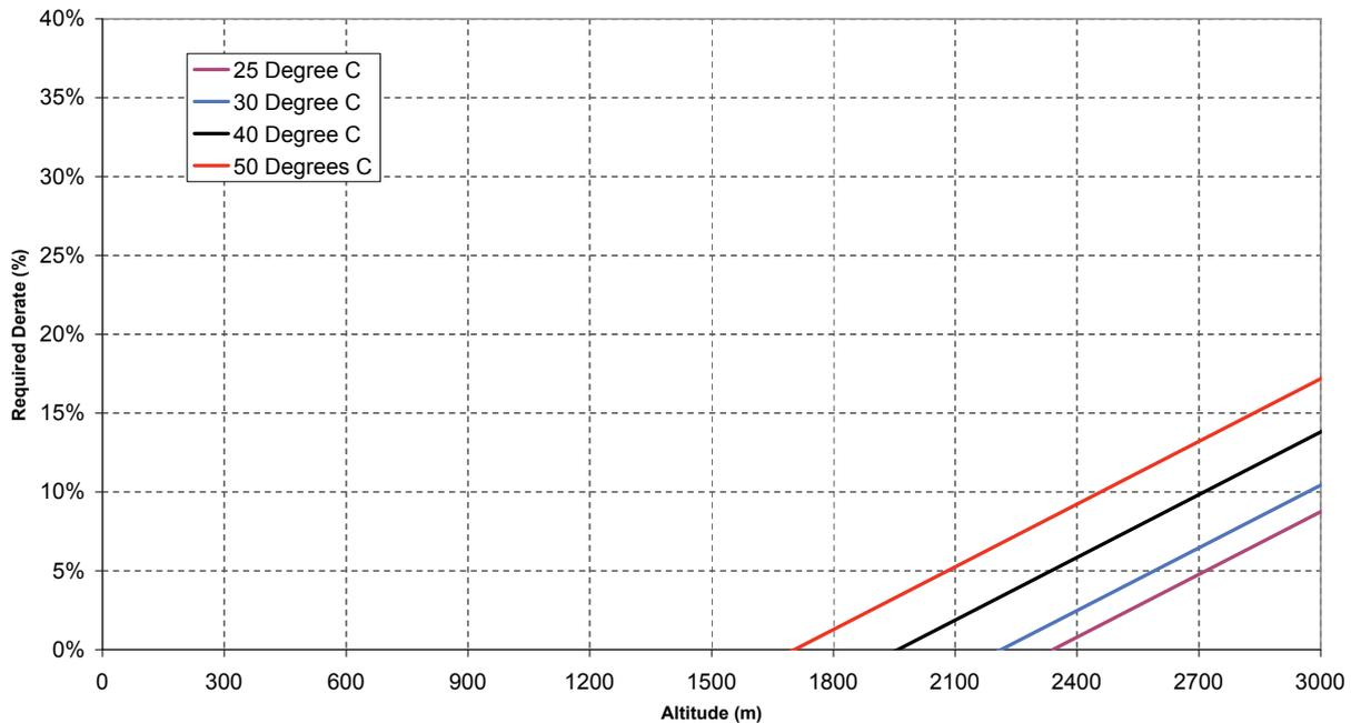
**Note:** Ambient temperature at air cleaner inlet.
