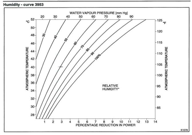
**Note:** When estimating the percentage reduction in power due to humidity, the relative humidity must be coupled with the ATMOSPHERIC AIR TEMPERATURE, and not the air inlet temperature which might be locally heated. The effect of inlet air temperature on power output must be considered separately using diagram 3952.
