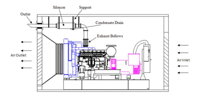
**Typical Exhaust System Installation.**
