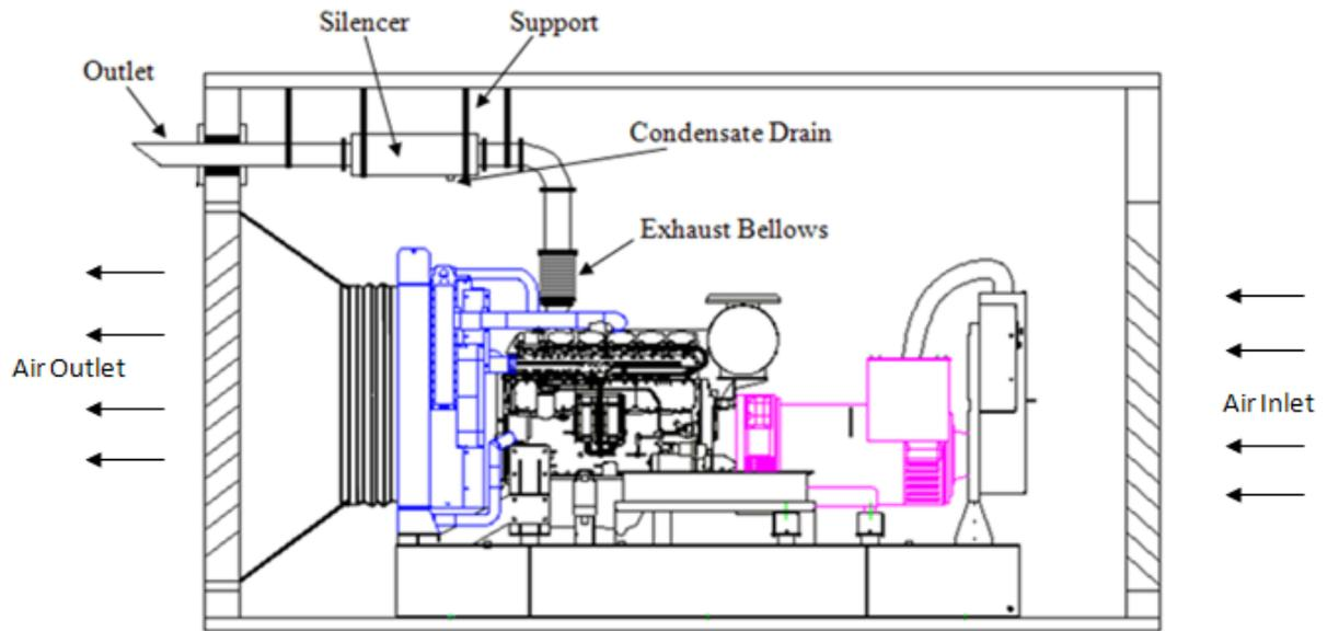
**Typical Exhaust System Installation.**
